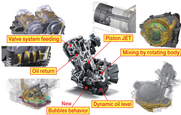
Fig1. Examples of oil behavior simulation using Particleworks
